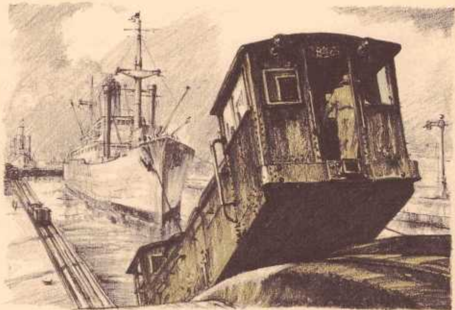
Locomotives, often called "mules," tow ships through the locks
